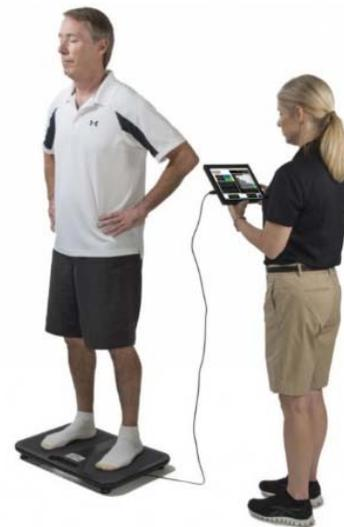
*Figure 2. Depiction of the BBT setup. Participants stood with eyes closed, hands on hips and two feet on the BTrackS™ Balance Plate, while BTrackS™ Assess Balance software guided the test administrator through measurement of COP path length over four trials.*
